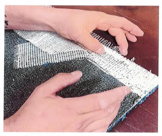
Run a bead of latex on the edge of the backing, then fold the weft yarns into the latex.
