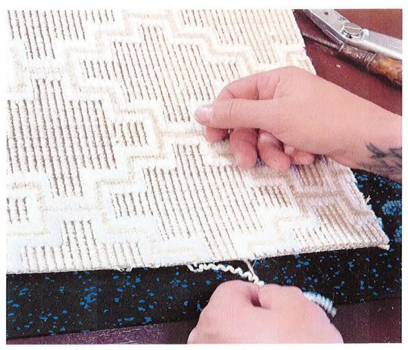
Using an awl or needle, deconstruct the seam edge by pulling the warp yarn, filler, and chain stitches, one at a time.
