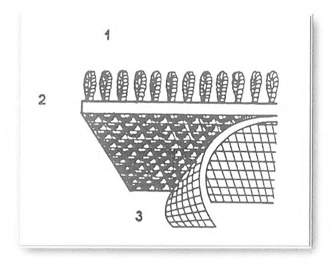
**Tufted Carpet** – In this form, tufted carpet is pile yarn pushed through primary backing and given body and stability by latexing the primary backing to the secondary backing. Pile can be level loop, cut pile or many combinations.
