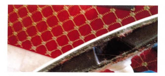
**Example of Improper Vacuum:** This picture illustrates what a beater bar vacuum will do. Should use suction only vacuum without a brush. Although this can be corrected with a tip shearing machine.
