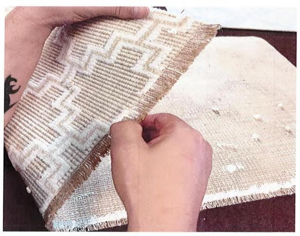
Push the latex through the weft yarns from the back, then pinch the latex through the weft yarns from the front, completely encapsulating the chain stitch.
