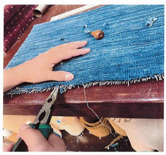
Using an awl and pliers, begin deconstructing the seam edge, exposing 1 1/2 inches of weft yarn.
