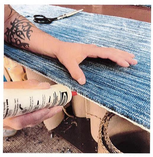
Run another bead of latex, making sure the chain stitch is completely encapsulated.
