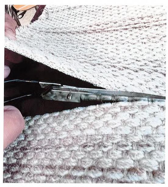
Cut the seam edge with a sharp pair of shears down the warp row without cutting any of the chain-stitch
