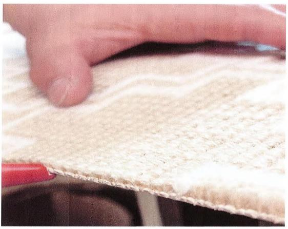
After cutting off the weft yarns, run another bead of latex on the edge.
